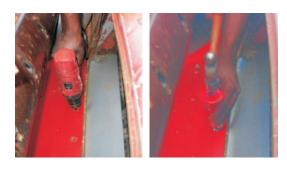
7. Using the remaining pre-drilled holes as a guide, drill thru the floor of the header with the 9/32" drill bit supplied.
