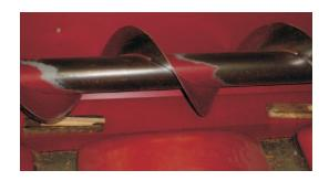
13. Wedge the panels tight against the bottom of the trough with the wooden shims supplied.
