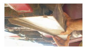
3. Remove the protective covers below the drive lines and gear boxes on the underside of the header.
