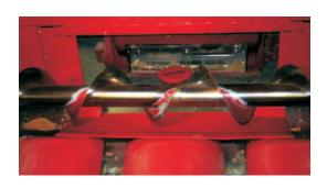
5. Insert the poly center panel under the auger as illustrated.
